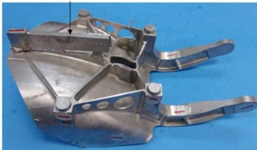
Figure 7. A casting showing an integrally cast test coupon. (Artwork courtesy of Uni-Cast, LLC.)
