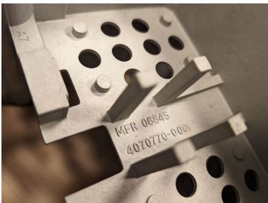
Figure 3. An investment casting showing cast finish and as-cast lettering raised. (Artwork courtesy of Uni-Cast, LLC.)
