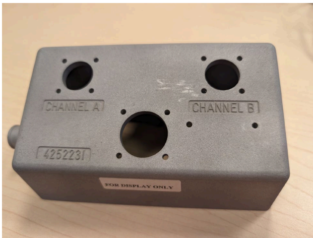
Figure 2. An investment casting showing cast finish and as-cast lettering raised in a recessed area. (Artwork courtesy of Uni-Cast, LLC.)
