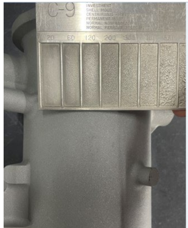
Figure 9. A C-9 cast microfinish comparator recommended for the evaluation of as-cast surfaces by the comparison method. (Artwork courtesy of Impro Aerotek USA, Inc.)
