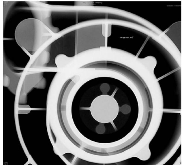
Figure 10. An x-ray of a production casting. (Artwork courtesy of O’Fallon Casting.)
