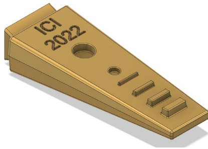
Figure 13. A rendering of the wax pattern produced from the AM die. 9
