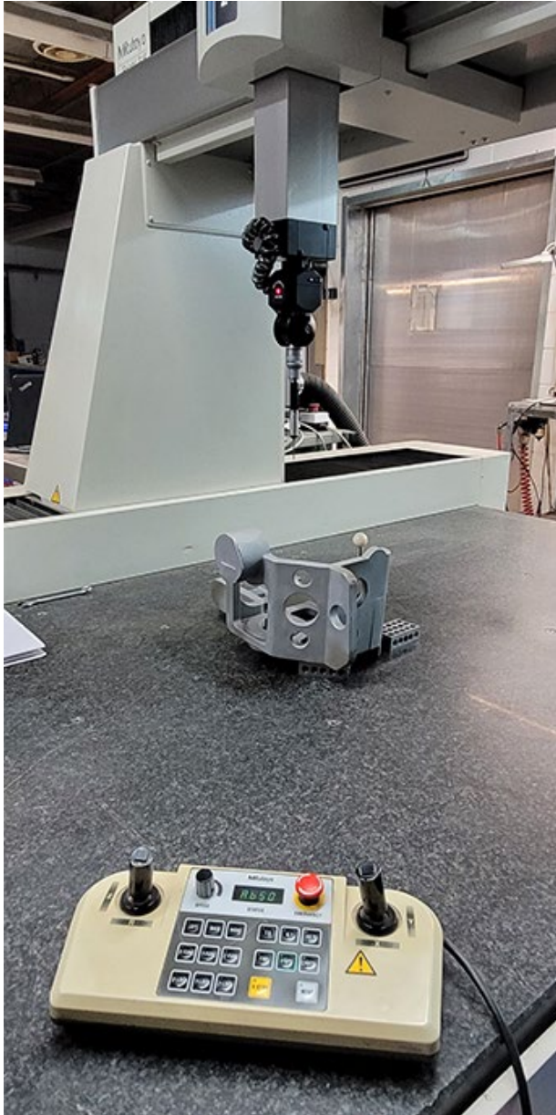
Figure 8. A casting undergoing dimensional inspection. (Artwork courtesy of Designed Precision Castings, Inc.)
