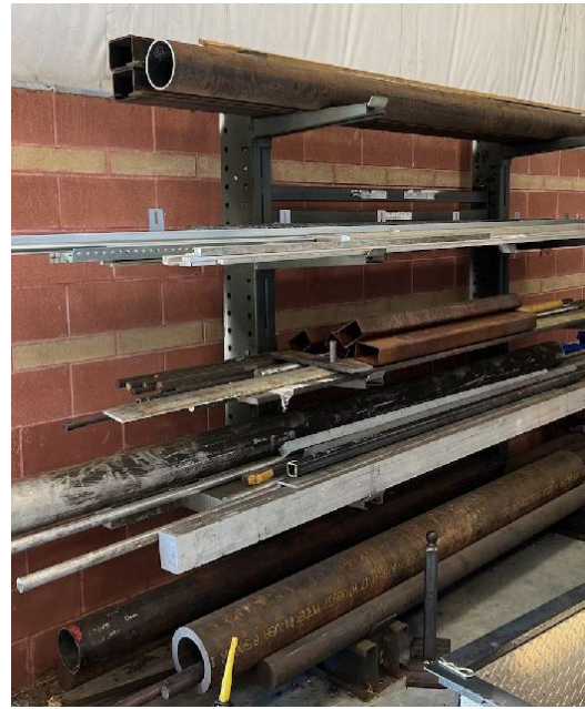
Figure 6. Barstock at a machine shop. (Artwork courtesy of Seco Machine.)
