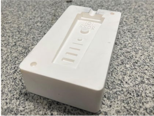
Figure 12. An example of a part of a die for making a wax pattern produced by Additive Manufacturing. 9
